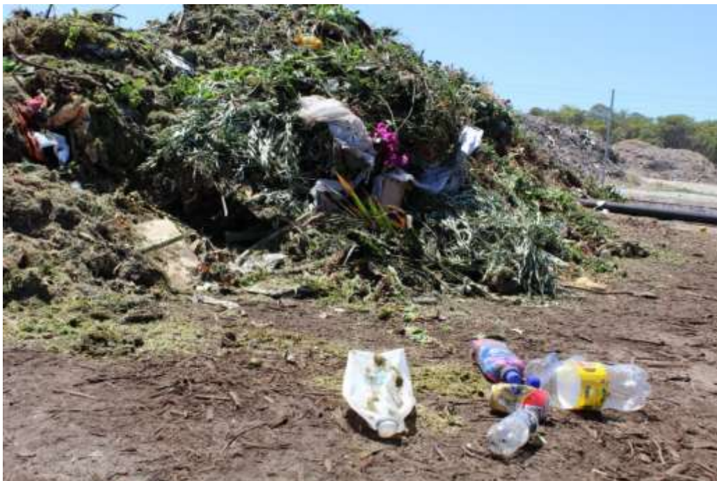
Figure 7: Plastic, glass and metal containers contaminate organic waste at Bunbury-Harvey Regional Council's composting facility
